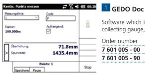
Software which is used in combination with the track measuring trolley GEDO CE 2.0 for collecting gauge, cant and twist paramteters.
